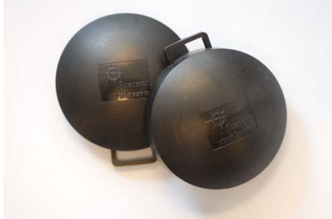
Figure 1: Passive etched track radon detector holders from Norwegian Radiation Protection Authority.
