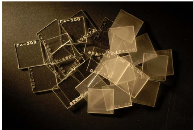
Figure 2: Passive CR-39 etched track radon detector films from Norwegian Radiation Protection Authority. Normally exposed films to the left and overexposed films to the right.
