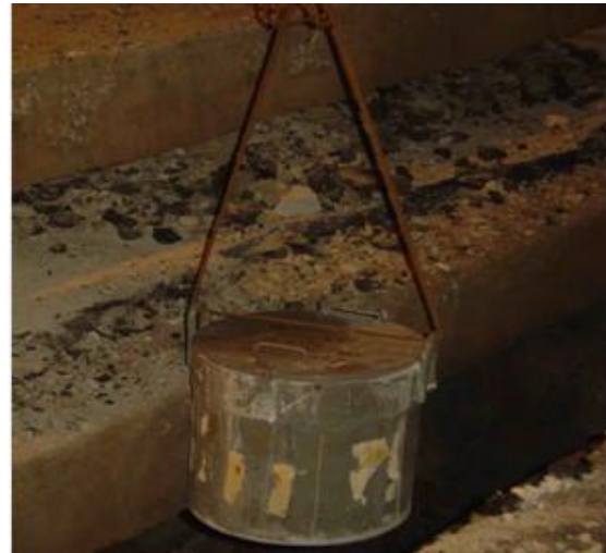
Fig.7 Conditioned DSRS in one of the canyons in the Point of Radioactive Waste Disposal (PRWD).
