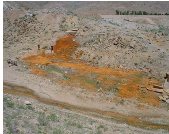
Fig. 9 Bottom sediments of the drainage waters stream of the Charkesar-2 mine. (Source SISIM, Uzbekistan)
