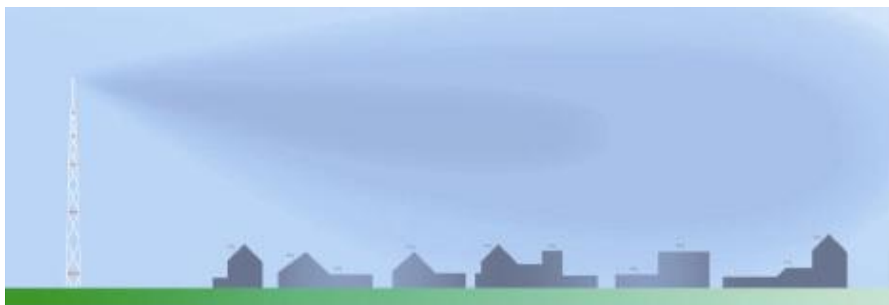
Fig.1. Radiowaves from mast-mounted antennas surpasses the people living in the vicinity of the mast.
